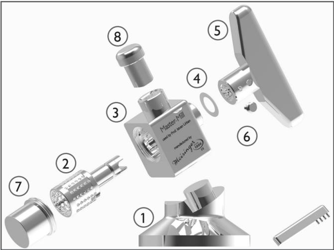
After processing, the individual components of the Master-Mill are assembled as follows:
